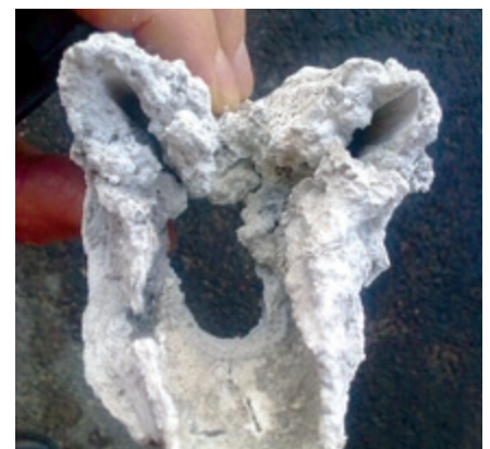
Urea deposit problems have become frequent and critical, considering that Stage 3B/Tier 4i regulations require cold and hot NRTC cycles.
