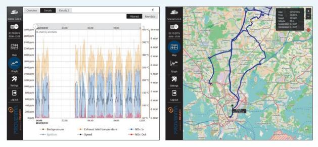
With the Proventia PROCARE<sup>™</sup> Drive emissions monitoring system, vehicle emissions can be reliably monitored and reported.
